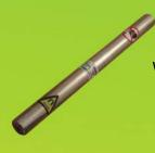
We produce magnetic rods in two different diameters (Fi 25 and Fi 34 mm), and in a length which our customers requires. We can put inner or outer thread on the sides of the pipe. The rods are filled with rare earth Neodymium N52 magnets, with a magnetic strength of Brmax=14 800 Gaus.
